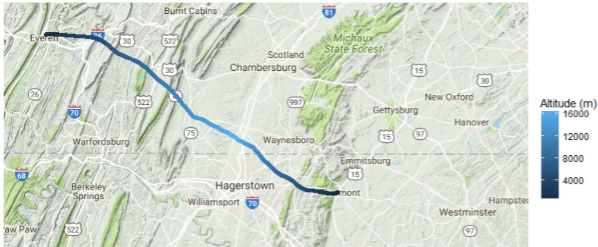
Chase was a wild ride! The tracking vans drove through winding pathways, trying to stay under the balloon to keep radio lock as the balloon entered the jet stream. The balloon continued upwards at a fast pace (6m/s) and then an as-yet-unexplained anomaly occurred: the balloon burst prematurely at 54,000 ft (as opposed to our expected 90'000 - 100'000 feet)! Perhaps a flaw in the skin of the balloon caused an early burst but currently, there is no conclusive evidence.
