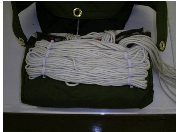
Figure 5 – Deployment Bag with Lines Stowed
