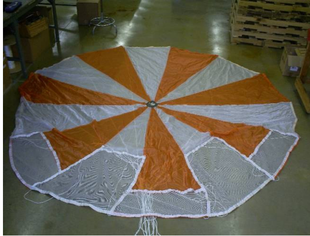
Figure 2 – Test parachute with "T-U" modifications
